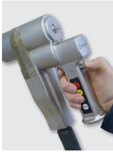
One-hand operation through integrated remote control and pneumatic control via handle
